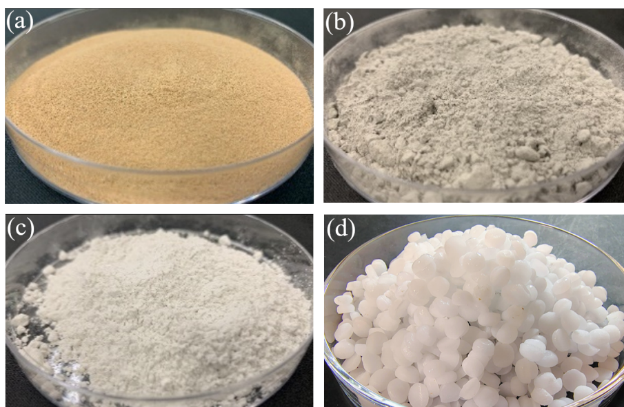
Figure 3.7. Materials used in testing (a) base soil, (b) ash, (c) slag, and (d) NaOH pellets used in this study
