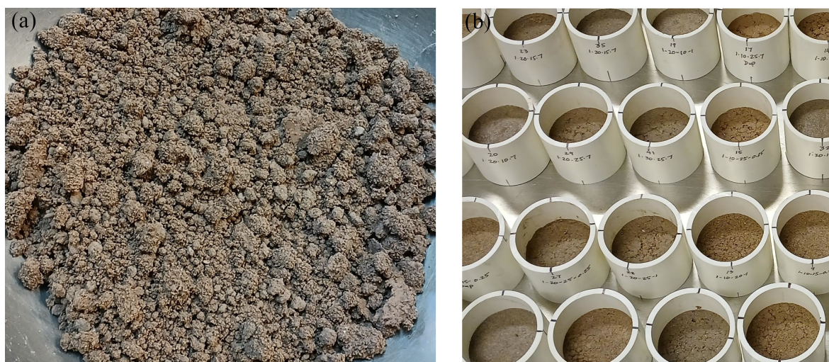
Figure 3.11. (a) Sample mixture after addition of the alkaline activator and (b) prepared specimens prior to wrapping in cling wrap and curing
