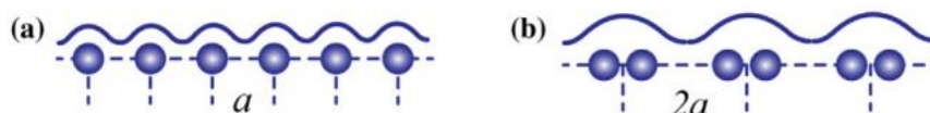
Figure 1.8: The schematic diagram illustrates the (a) one-dimensional chain and (b) two-dimensional lattice chain with dimerization. The change represents Peierls phase transition affect in atomic scale. 50
