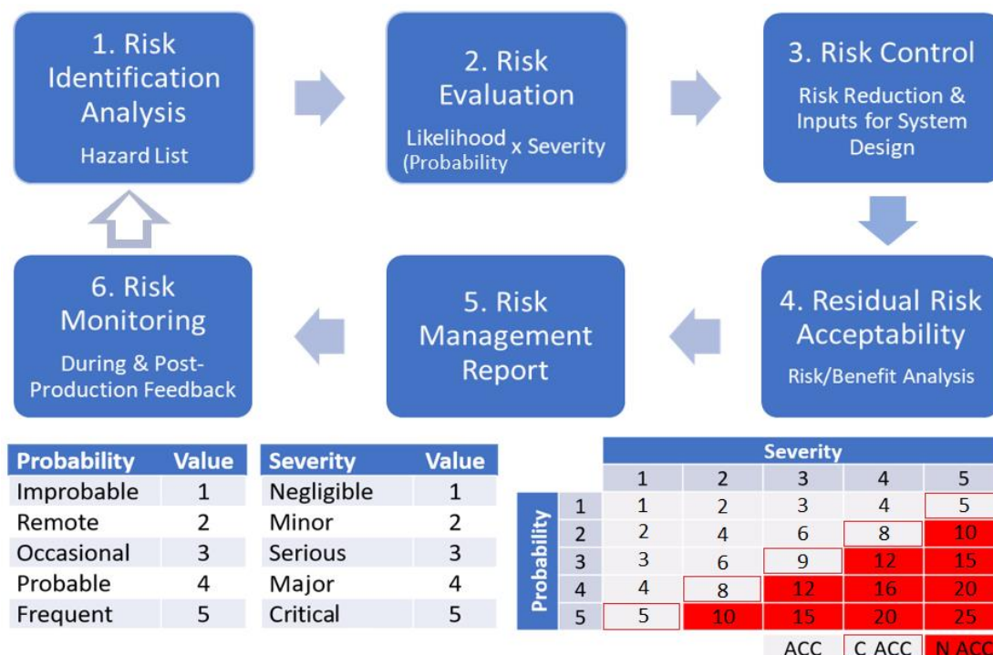
Figure 4.2. Semi-quantitative risk matrix calculated from the estimated probability and severity of risks with the six key stages of the ISO 14971 risk management process [241, 243, 244]. The probabilities are scaled from between 0–1 (or estimated based on the descriptor) to multiply with the severity rating and produce the risk matrix table with risk priority number (RPN) outputs in the range of 1–25. ACC = Acceptable; C ACC = Concern for Acceptance; N ACC = Not Acceptable.
