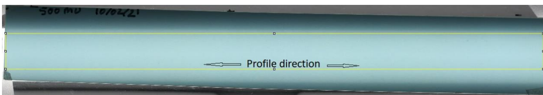
Figure 5-3 : Selection of a rectangle in ImageJ to create a profile along the short side of scanner.
