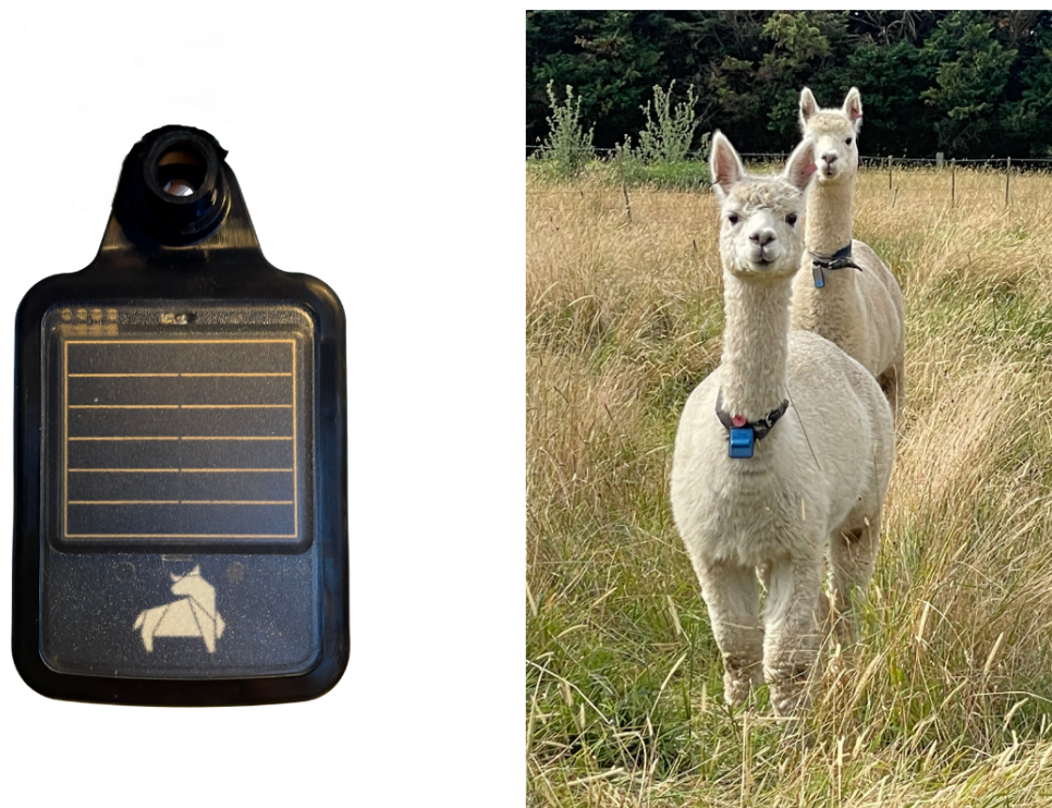
Figure 1. Smart Paddock Bluebell tag with prominent solar panel (left) and the collar with tag on the treatment group alpacas (right).
