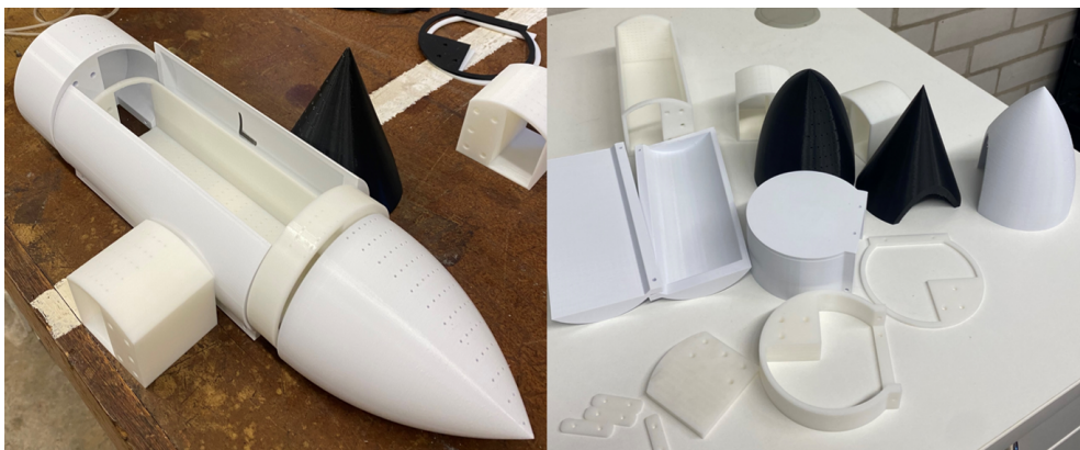
Figure 3.10: Fuselage Cavity Model: 3D Printed Parts
