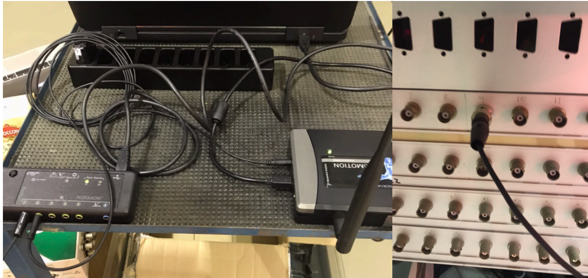
Figure A2.6: Noraxon Myosync connection to Receiver and MAS
