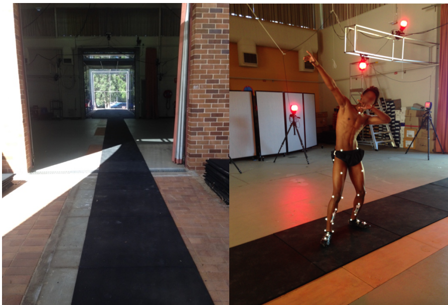
Figure 3.2: Overground track set up for Pilot testing the dorsaVi's ViMove IMU system (affixed to the lower leg) against the university's 3D Motion Analysis System (Eagle and Cortex 1.1.4.368, Motion Analysis Corporation, Santa Rosa, CA, USA)
