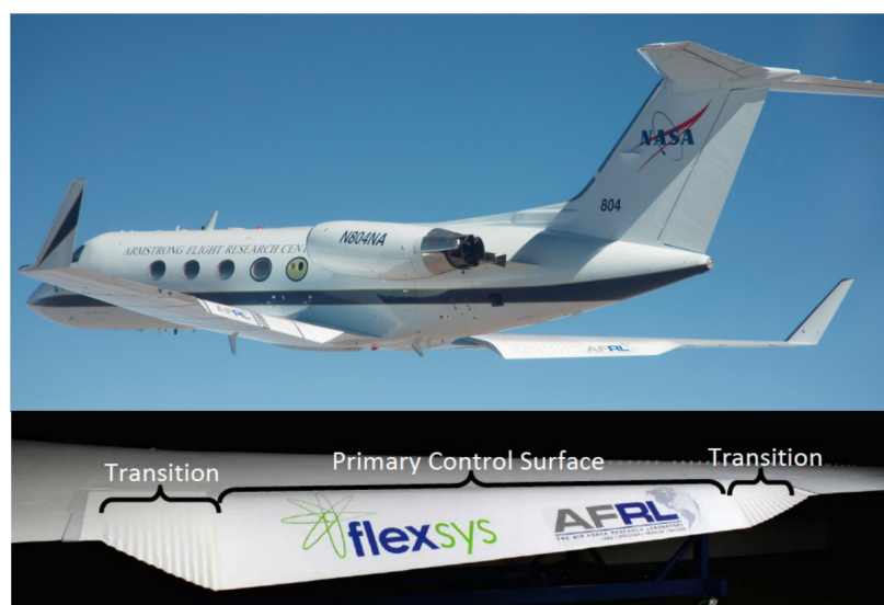
FIGURE 2.14. Flexfoil tested on the Gulfstream III business jet [12]
