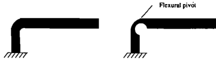
FIGURE 2.15. Definition of distributed compliant mechanism and lumped compliant mechanism[18]
