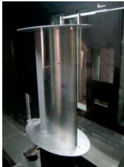
FIGURE 2.12. MACW aluminium model installed in SARL facility [10]
