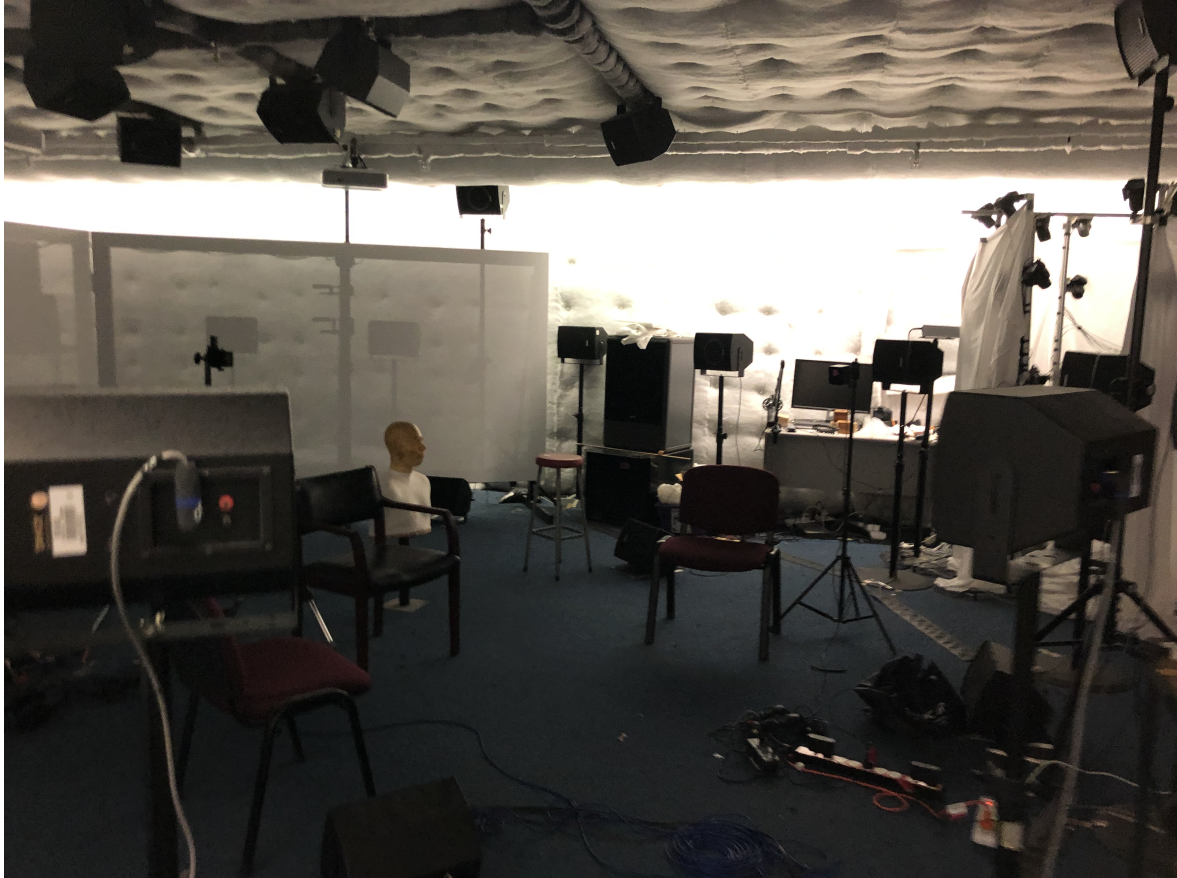
FIGURE .7. A photo of the place taken for the listening test. We took our subjective listening tests in the Carlab (Computed Audio Research Lab) at Electrical and Information Engineering at the University of Sydney. The participants were asked to listen to sit on a chair and put on a headphone (AKG K52) before starting the test. They were encouraged to adjust the volume to ensure the sound levels were appropriate to their hearing. The computer played each sound at a time, and the participants were asked to rate their preference for the sound.
