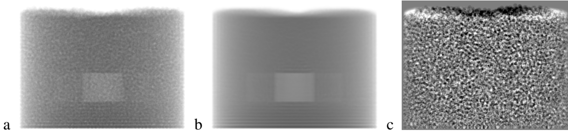
FIGURE 4.9: Artificial radiograph for 3 mm glass beads along the normal to X-axis showing: a) Measured X-ray intensity I_f of the container; b) Mean intensity \text{avg}(I_f) ; c) Normalised intensity \log\left(\frac{I_f}{\text{avg}(I_f)}\right) used for deconvolution.
