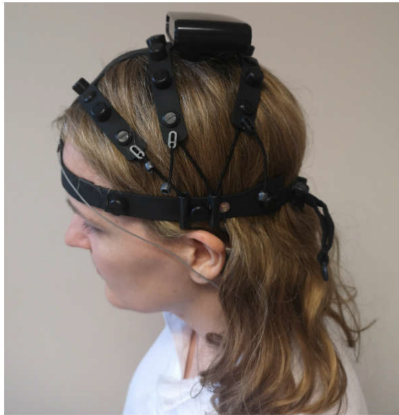
Figure 2.2: aEEG devices offer compact, portable solutions for long-term brain monitoring, enabling EEG signal acquisition outside of traditional hospital settings. However, the design of the headset does not yet provide sufficient comfort for long-term wear. Adopted from [21], licensed under CC BY 4.0.
