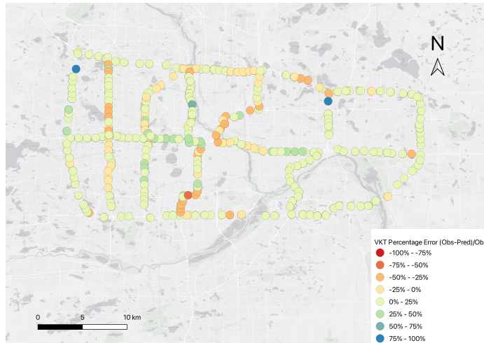
(B) VKT Percentage Error at Each Loop Detector station for Soft Voting
