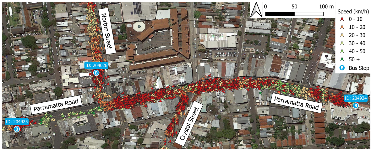
FIGURE 5.4: GTFS-Realtime Vehicle Positions data at the intersection of Parramatta Road and Norton Street, Leichhardt, Greater Sydney, Australia. Due to the proximity of a bus depot to the north of Norton Street, many buses make right turns at this intersection. During the morning peak, heavy eastbound traffic towards the city leads to significant speed reductions for right-turning vehicles, including buses.
