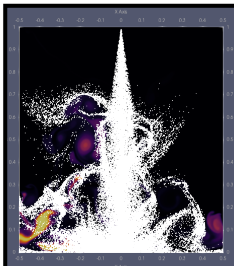
Figure 7-9: The water spray has successfully reduced the fire's size
