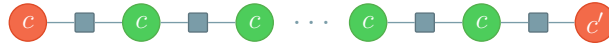
Fig. 4.5 If all the checks commute, then the value of the ancillary bit has to coincide with c . In this sense, the repetition code allows for the value c to ‘travel’ through space.
