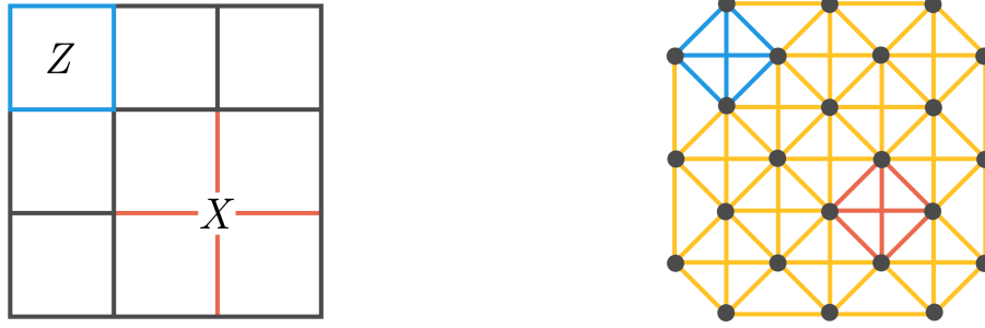
Fig. 3.5 Comparison between a patch of surface code (left), with the resulting connectivity graph (right). The Z and X stabilisers highlighted on the left result in the edges highlighted in in the right picture. From [31].
