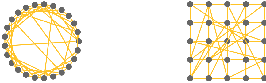
Fig. 4.1 A well connected graph (on the left) tends to induce very long edges when embedded in 2D [32].
