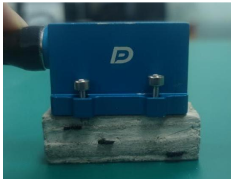
Figure 3-31. Experimental setup for ultrasonic phased array testing.
