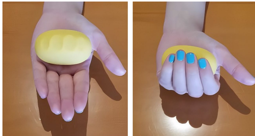
Figure 3. Squeeze ball dynamometer (Smart Stress Ball, 2019 China) used by participants to record daily grip strength to their smartphones via Bluetooth.
