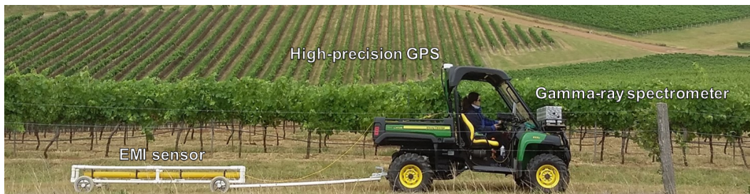
FIGURE B1. On-the-go Dual EM-21S electromagnetic induction (EMI) meter (Dualem Inc., Ontario, Canada) and RSX-1 gamma-ray spectrometer (Radiation Solutions Inc., Ontario, Canada) can be used as part of a multi-sensor platform to map soil moisture content and salinity (via EMI), and soil type and parent material (via Gamma). Together, these complementary sensors can be used to map patterns of soil variability, alongside a high-precision GPS unit mounted to the vehicle.
