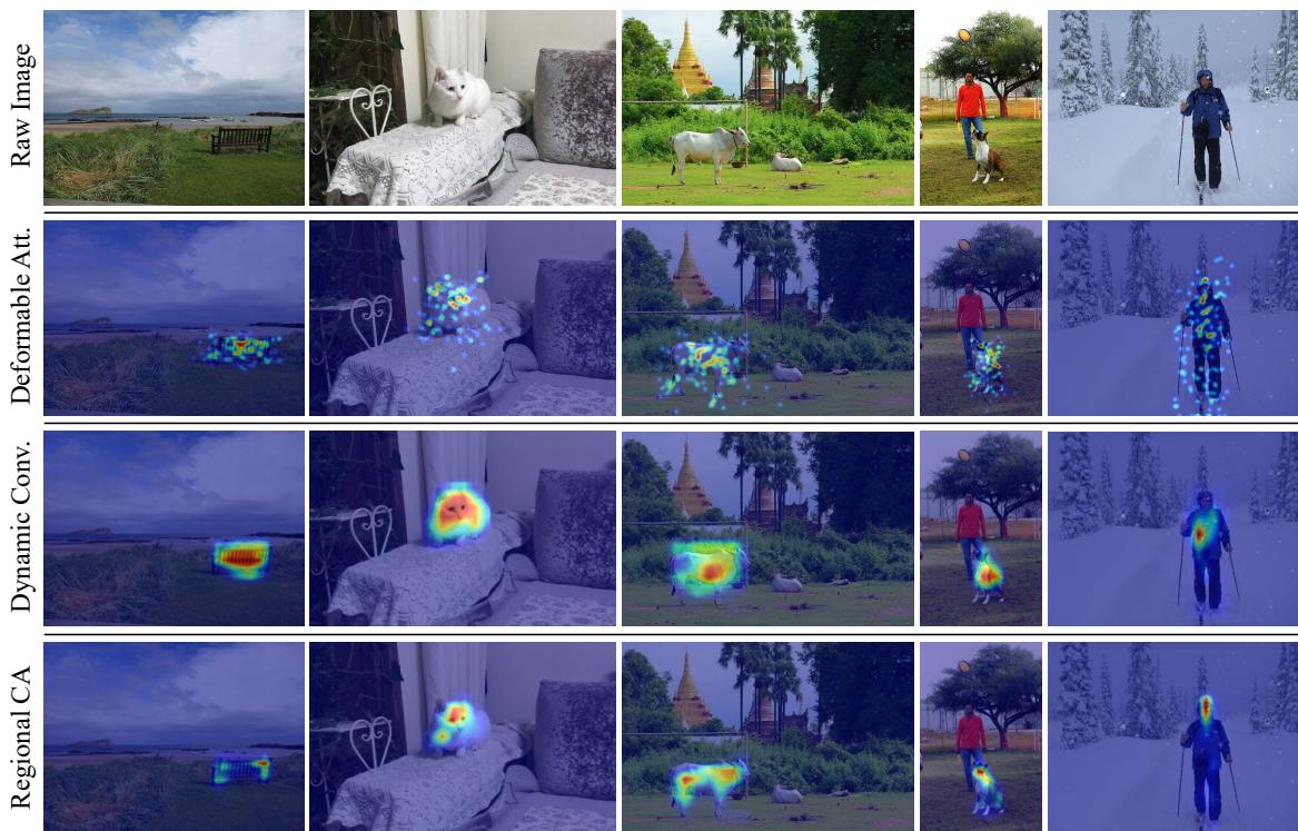
FIGURE 3.5. Visualizations of the activation maps for deformable attention (the second row), dynamic convolution (the third row), and regional cross attention (the last row).
