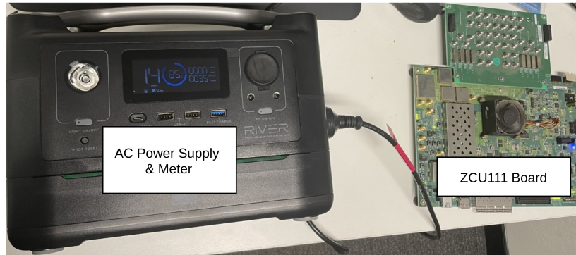
FIGURE 3.19. Measuring the power consumption of the ZCU111 via AC power supply
