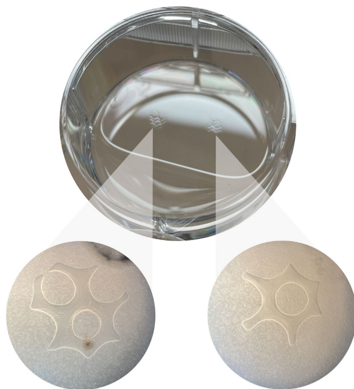
Figure 4.5 Micropatterning of PEG hydrogels on tissue culture plastic was achieved using photopolymerisation of a PEG prepolymer solution.
