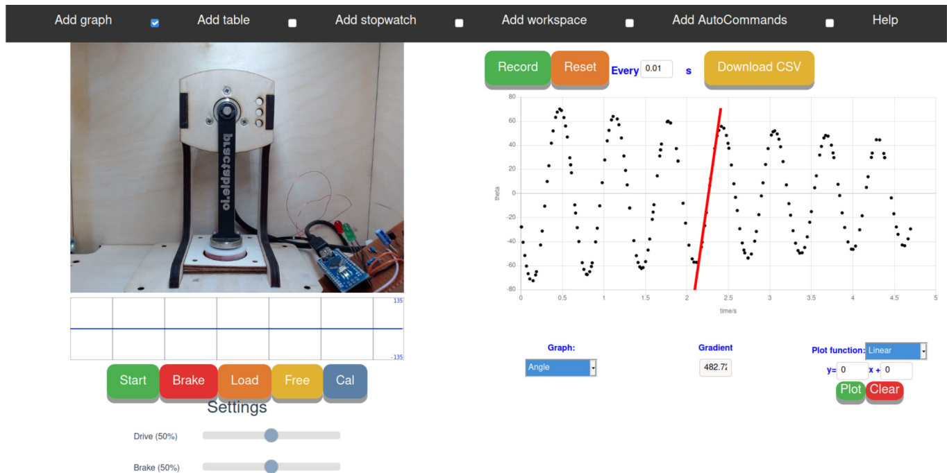
Figure 2: Screen grab of the ‘pendvueino’ remote lab interface with graphing tools including graphing different quantities, gradient calculation tool and function plotter.
