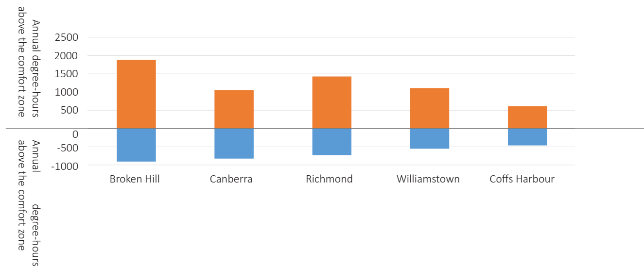
Figure 2.36: Annual number of degree-hours of discomfort Annual number of degree-hours of discomfort above (red) and below (blue) the comfort zone
