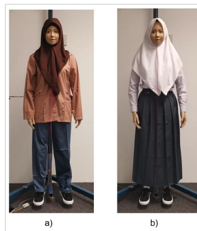
Figure 3.2 Ensembles with the lowest and highest clothing insulation. a) Ensemble C3 has an intrinsic clothing insulation of 0.73 clo; b) Ensemble A.2.2 (with legging) has an intrinsic clothing insulation of 1.08 clo
