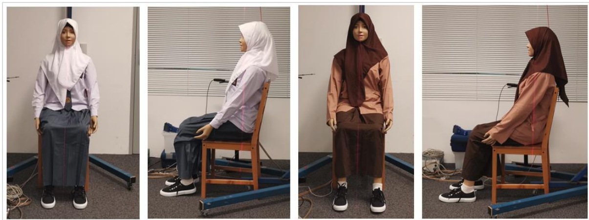
Figure 3.3 Sitting position on a wooden stool mimicking Indonesian classroom chairs. The stool was elevated during measurements to prevent conduction effects by ensuring the soles of the feet do not touch the floor.
