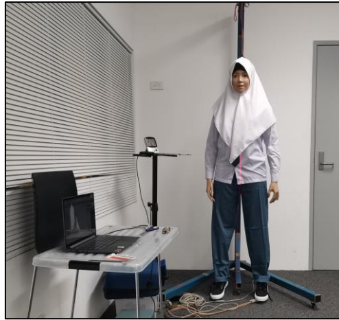
Figure 2.6 Laura Palmer, female thermal manikin at IEQ Lab, The University of Sydney
