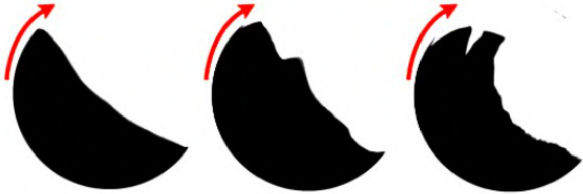
FIGURE 4.1. Schematic of different powder flow conditions as measured by the Granudrum, with drum rotation in the direction of the arrows. On the left, powder has a low velocity angle, as seen by the shallow slope of the powder face, and also has a low cohesion value, as seen by the uniformity of the powder face. These are indicative of good powder flow. Powder flow worsens towards the right, with a steeper velocity angle and a wider face indicating worsening powder flowability. Figure is reproduced from the Granudrum user manual [265].
