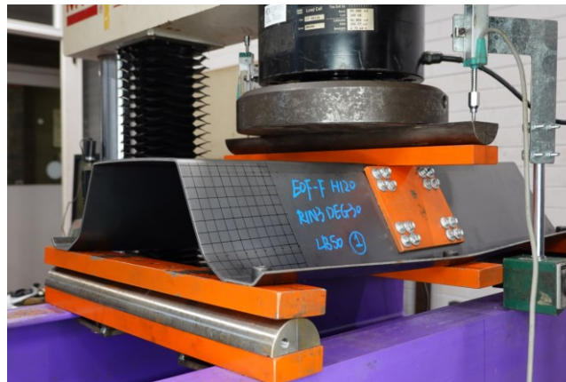
Figure 61 flexural failure followed by web crippling
