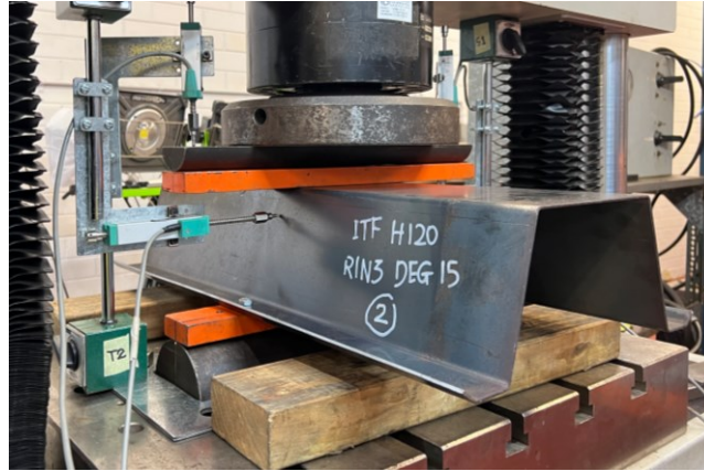
Figure 40 ITF loading case setup
