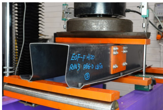
Figure 58 Typical failure mode of vertical web sections with small RIN for EOF-F loading case
