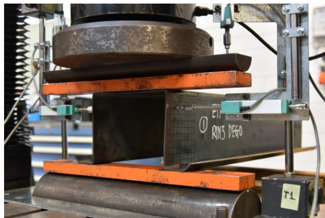
Figure 67 Typical experimental setup for ETF loading case
