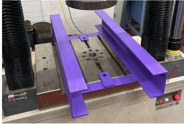
Figure 42 Test rig for OF loading cases
