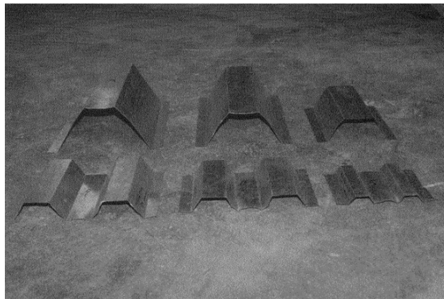
Figure 32 single and double ribs hat sections tested by Wu et al. [16]
