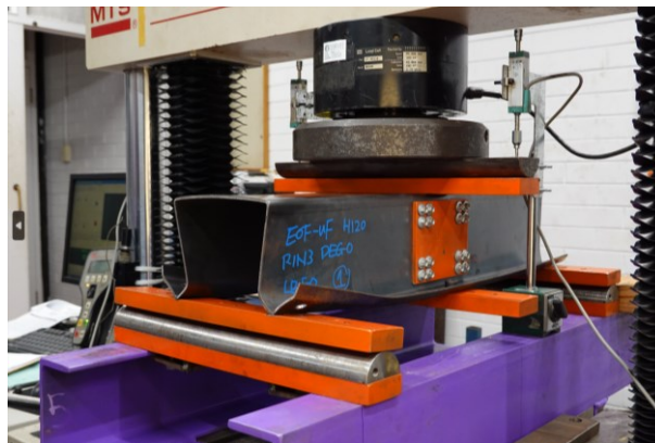
Figure 97 Asymmetric failure at two ends for EOF loading case, experimental study photo
