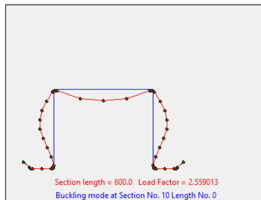
Figure 23 Buckling shape for ITF-F-H120-RIN3-DEG0-N50 at Section No. 10
