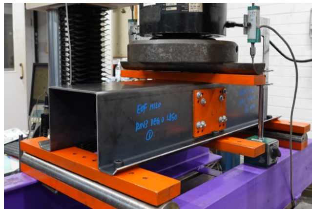
Figure 74 Typical experimental setup for IOF loading case
