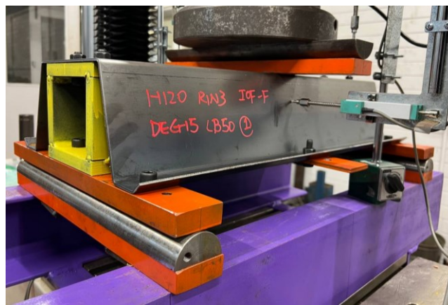
Figure 43 Assembly with bearing plates (IOF loading case) including half rounds and specimen
