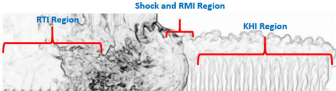
FIGURE 2.5. Simulated flow in Rotating Detonation Engine combustion chamber as the detonation wave progresses through the injected fuel and the consequential disruption to the shock due to the lag in fuel and oxidiser mixing [19].
