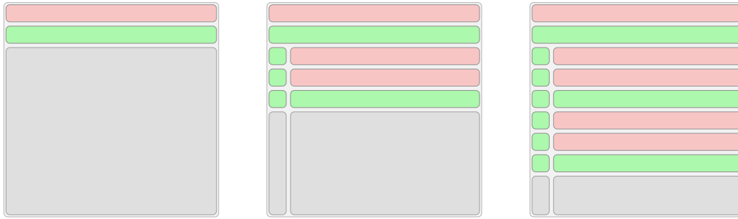
(a) Initial register placement, (b) Second and third register placement, following register allocation rule 1. (c) Continued allocation using register allocation rules 4 and 5. Allocation halts at this point as the number of registers allocated to the QCB satisfies the number of registers required by the DAG.
