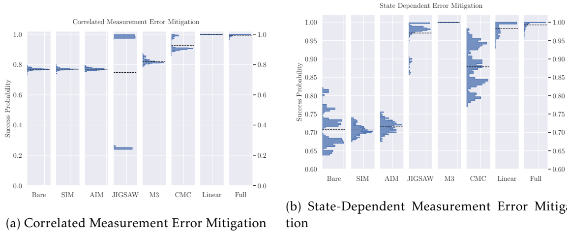
Figure 6.10: (a) A sample correlated measurement error mitigation. (b) A sample state-dependent measurement error mitigation. Dashed lines indicate the average of each distribution. The ‘Bare’ column shows the error distribution without before any mitigations are applied. The bifurcation of JIGSAW occurs where due to the pathological nature of the error model the sub-tables may be missing entries, leading to errors during renormalisation.
