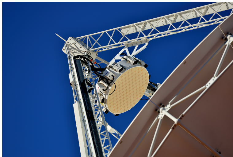
FIGURE 1.7. ASKAP phased array feed (PAF) at the focus of an antenna, Credit: CSIRO
