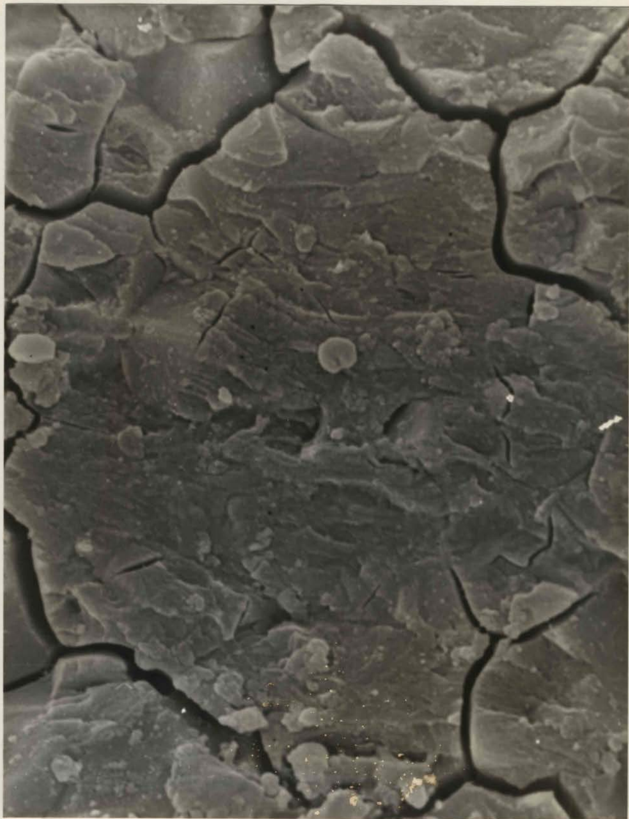
Plate 8. Scanning electron micrograph of an area of translucent endosperm in a chalky cored grain of Kulu rice (X 4300)
