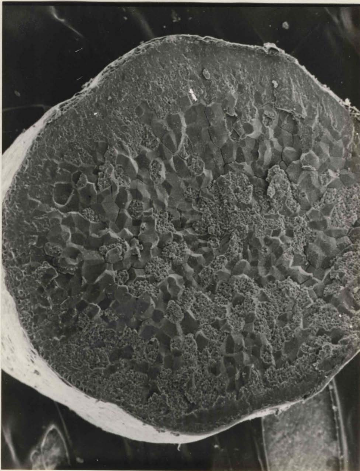
Plate 7. Scanning Electron Micrograph of the naturally suncracked surface of a chalky cored grain of Kulu rice (X 135)
