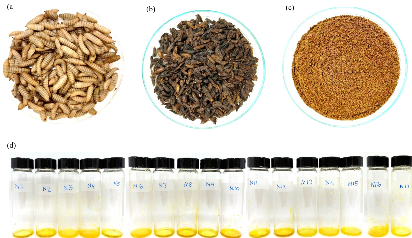
Fig. 4.6: Visual and physical properties of the BSFL; (a) Fresh BSFL which is approximately at ages of 14 days, (b) Dried BSFL which was dried at 60 °C for 48 hours, (c) BSFL has been ground finely and ready for the SC-CO 2 extraction, (d) Larvae Oil extracted with SC-CO 2 with various conditions of pressure, temperature and extraction time. CO 2 flow rate was constant with an average of 1.2 lpm.
