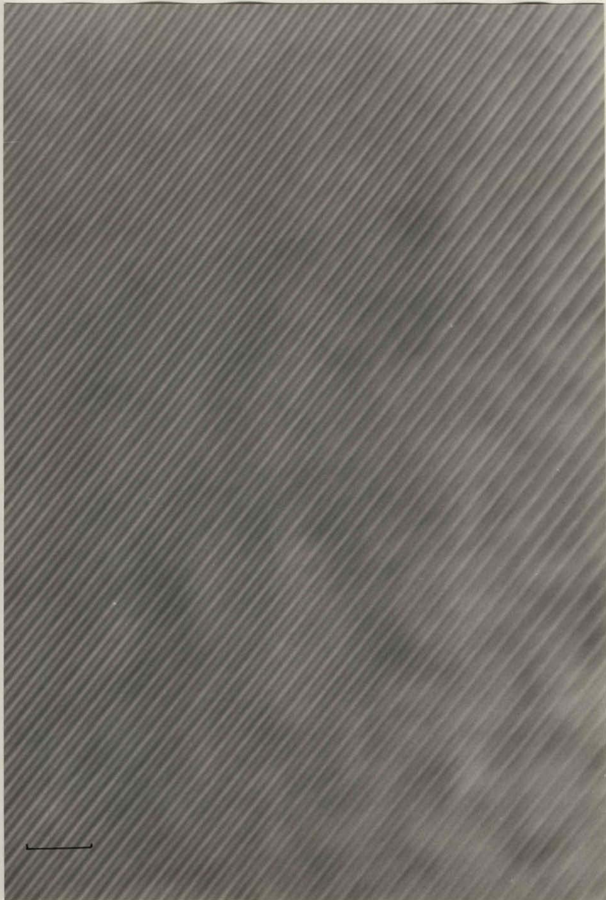
Plate A4.2. A HRTEM Z-axis image of relic pyroxene from the basement sequence in the Wilandra Inlier (sample 861314; scale bar 35 Å.). This plate presents an example of perfect "single-chain" structure of the crystal.
