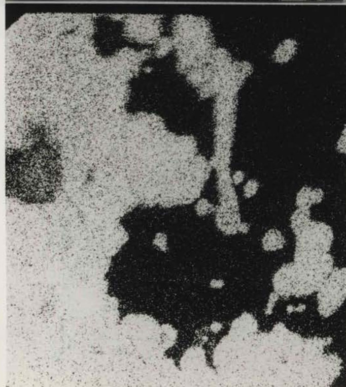
Plate A3.2. Compositional variation of cryptomelane and coexisting phases. The BSE images show that the cryptomelane is K- and Mn-enriched, while the surrounding dark grey areas in Plate A.3 are Fe- and Ca-enriched. x 400; sample SD-12
