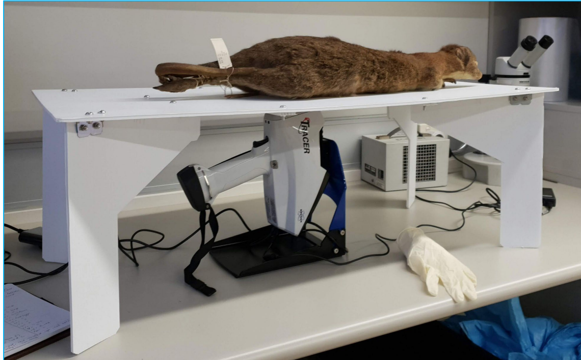
Fig. 2.6: The custom built specimen stage allowed the specimen to rest, fully supported above the pXRF spectrometer.
