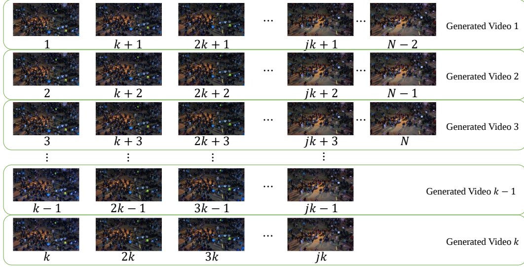
FIGURE 5.4. Illustration of multi-frame-rate dataset generation. We obtain k new videos with \frac{F}{k} fps given the original video with F fps.
