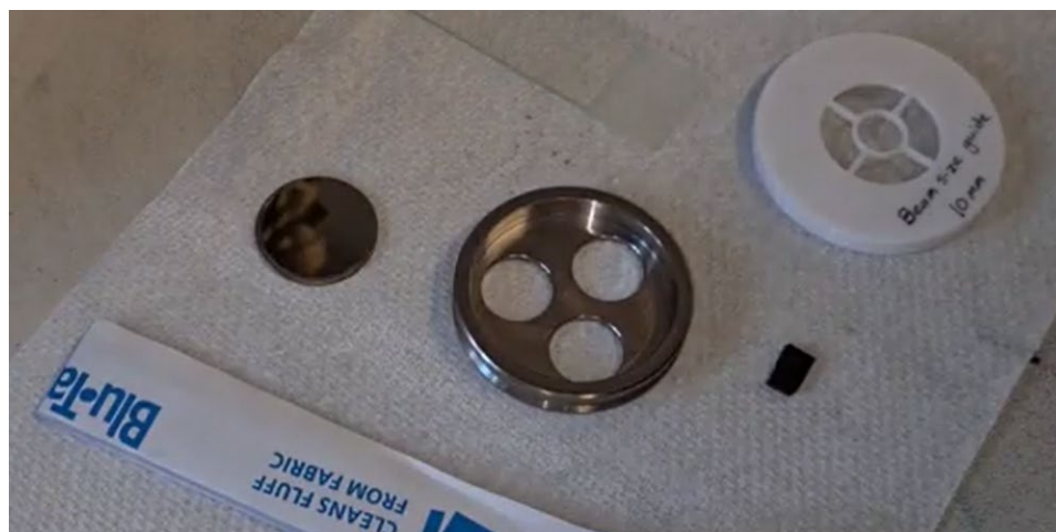
Fig 3-4. Items required for XRD instrument sample preparation.
