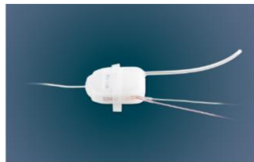
Figure 2-3 Picture of M series implant, an upgraded telemeter for data collection. 211
