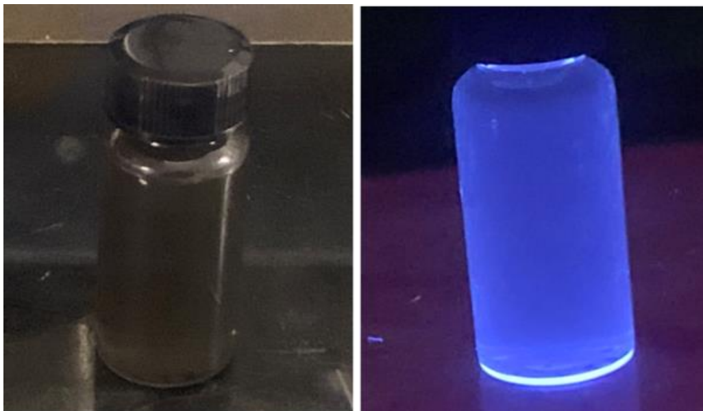
Figure 11 L-R, Microwave synthesized QD (a), and QD showing photoluminescence effect under 320nm light (b).
