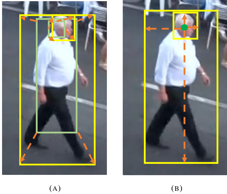
FIGURE 5.4. Illustration of our anchor-free approach vs. traditional static head-body ratio anchor-based approach. a). Anchor-based approach, where head and body boxes are regressed from separate RoIs. b). Our anchor-free approach, where head and body boxes are predicted simultaneously from the same grid box, achieving a faster inference speed and fewer parameters for training.
