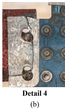
Figure 4.22: Deformation and fracture behaviour of the specimen T1.2-12-50-2.0-25-02 with RR=2.0
