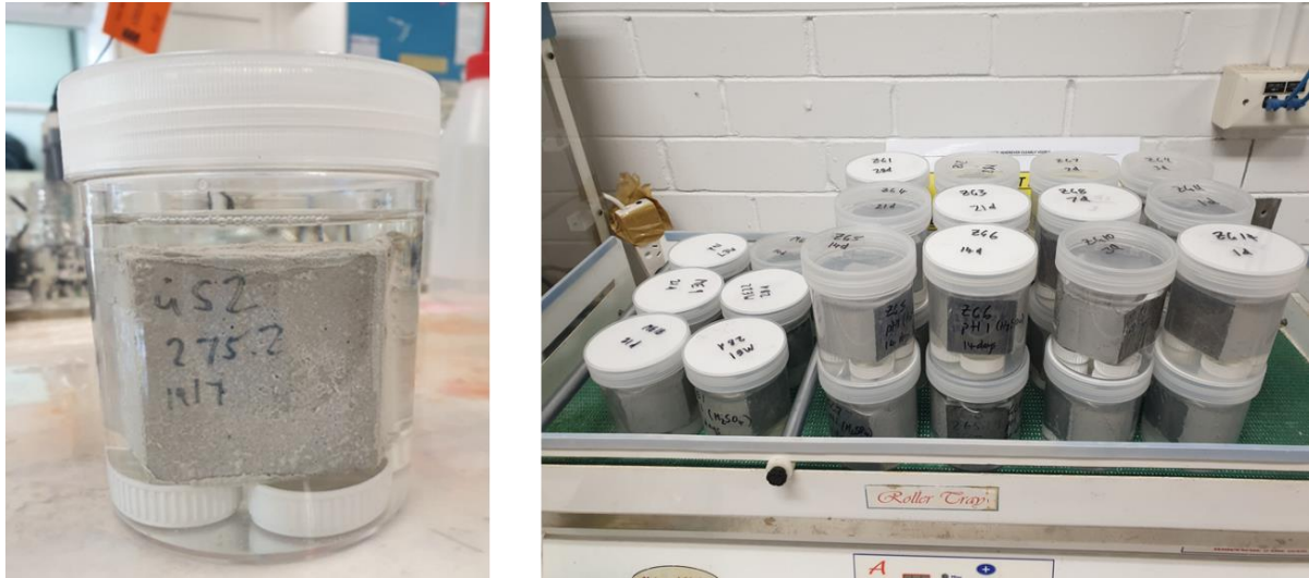
Figure 3-3 Accelerated corrosion test
