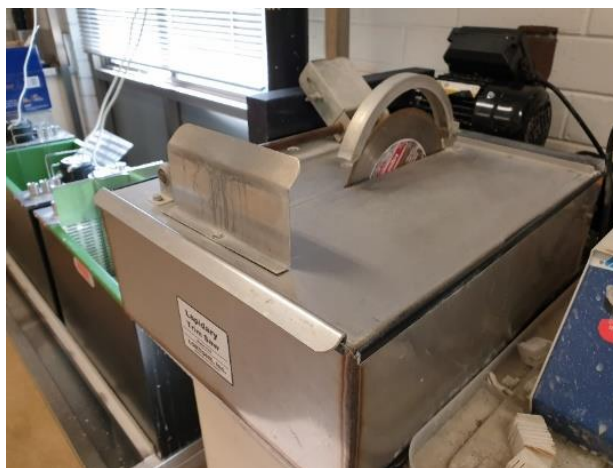
Figure 3-21 Lortone inc Model FS8 Lapidary Trim Saw equipped with an 8-inch diamond blade
