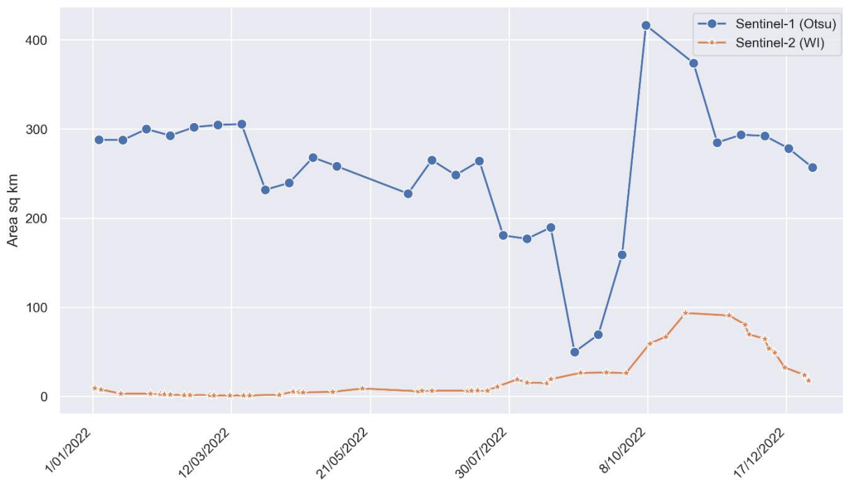
Figure 3.42: Figure showing discrepancy between area delineated using Sentinel-1 and Sentinel-2 in sq km.
