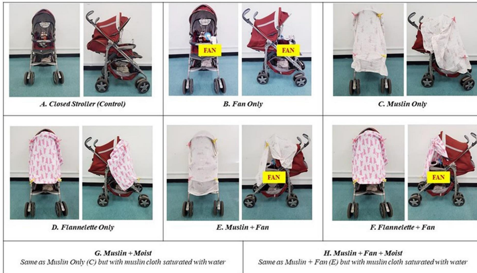
Figure 3. The tested stroller cooling interventions. All fabric drapings were secured using plastic clothes pegs, ensuring that there were no gaps present. For illustrative purposes, the drapings of interventions E and F were raised on one side to display the position of the battery-operated fan.
