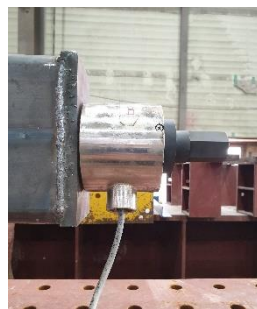
(b) Installation of load cell-1 & load cell-2
