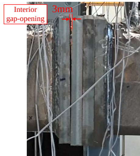
(a) Deformed shape with the interior gap-opening at displacement 34mm (drift 2.21%) with F_u = 140kN
