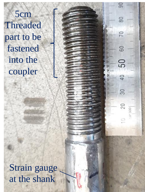
(b) Bolt thread in column-1F
