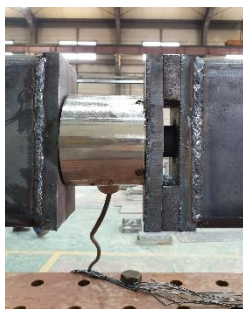
(b) Installation of load cell-1 & load cell-2
