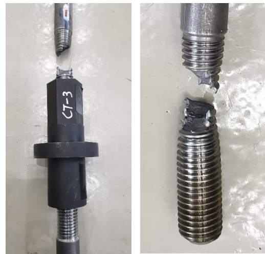
Figure 4.19: Load-strain curves of coupler & SRB and image of failure from uniaxial test
