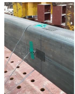
(c) Strain gauges on the SRB and the column
