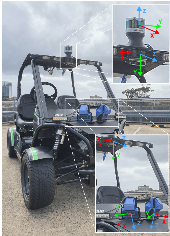
Figure 3.7 – Sensor setup. Top-right shows the coordinate frames of the VLP-16 and camera, and the bottom-right shows the frames of the two Baraja Spectrum-Scan sensorheads and camera. The Baraja Spectrum-Scan sensorheads had to be calibrated with the camera separately.
