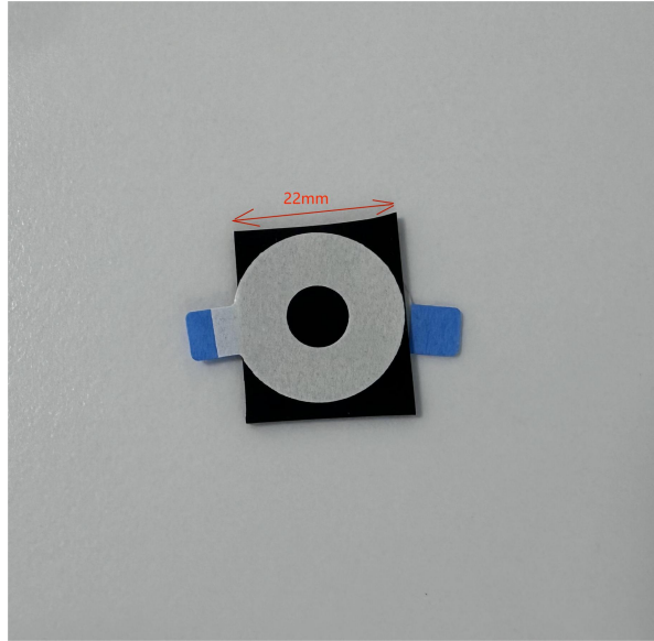
Figure 3.11: The adhesive washer on square rubber sheet
