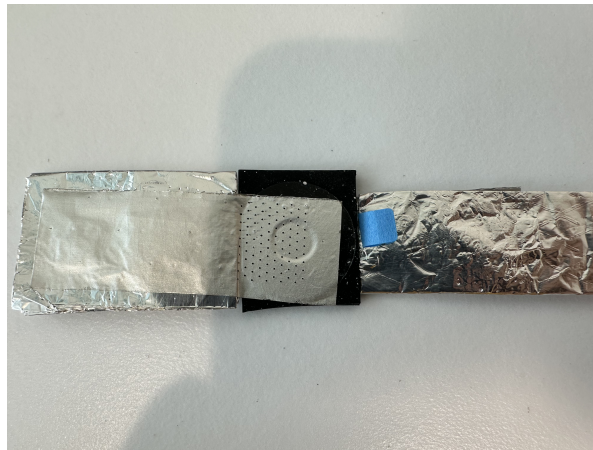
Figure 3.12: An adhesive washer and flexible electrode affixed to the opposite side of the rubber square
