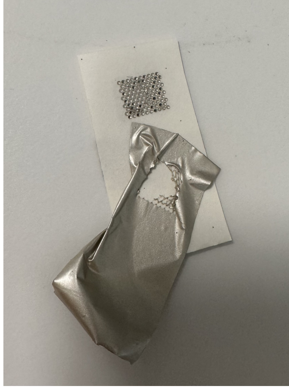
Figure 5.1: Broken Z-conductive Electrode with a Hole Spacing of 1.0 mm and a Hole Diameter of 0.75 mm.
