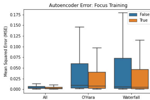
Figure 2.12 – Box-and-whisker plot highlighting the performance improvement when using focus training, where only patches with high loss are trained on. These results are with patch size of 21 \times 21 , where ‘True’ indicates focus training has been used, while ‘False’ indicates it has not.
