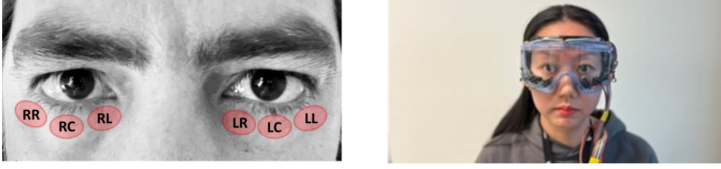
Figure 3.4: (a) The placements of NIRSense sensors under the eyes, 3 sensors on each side from left to right and are named as LL, LC, LR, RL, RC, RL based on their locations. (b) The photo of the participant wearing the NIRSense glasses on (The image is cropped to meet the anonymous review policy because an author’s face is included).
