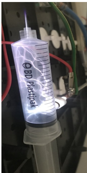
Figure 3.12: Photograph of a unused version of the plasma treatment vessel design from Figure 3.7D with the quartz plasma pen (O.D. 4 mm I.D. 2 mm) and the power supply was the commercially available NeonPro neon light power supply. The side port slipped so that the opening into the syringe body was semi-obstructed, resulting in this filamentary discharge.
