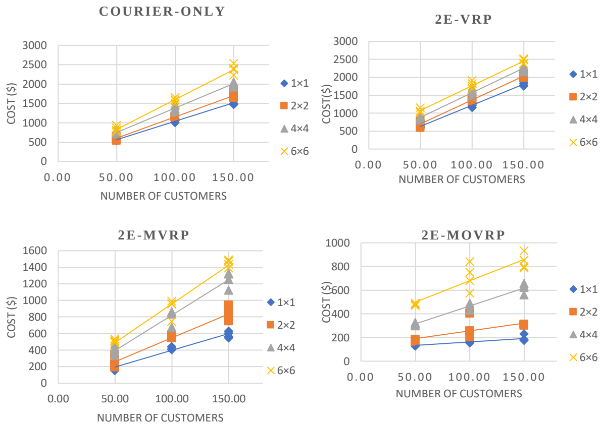
Figure 2.7. The objective value of 2E-MOVRP, 2E-MVRP, 2E-VRP, Courier-only algorithms in the networks with 50, 100, 150 customers
