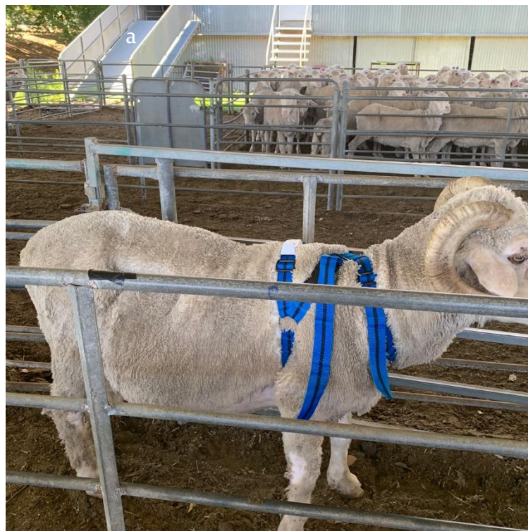
Figure 4.1: The Smart Tag (a) fitted posterior to the withers of a ram via a harness
